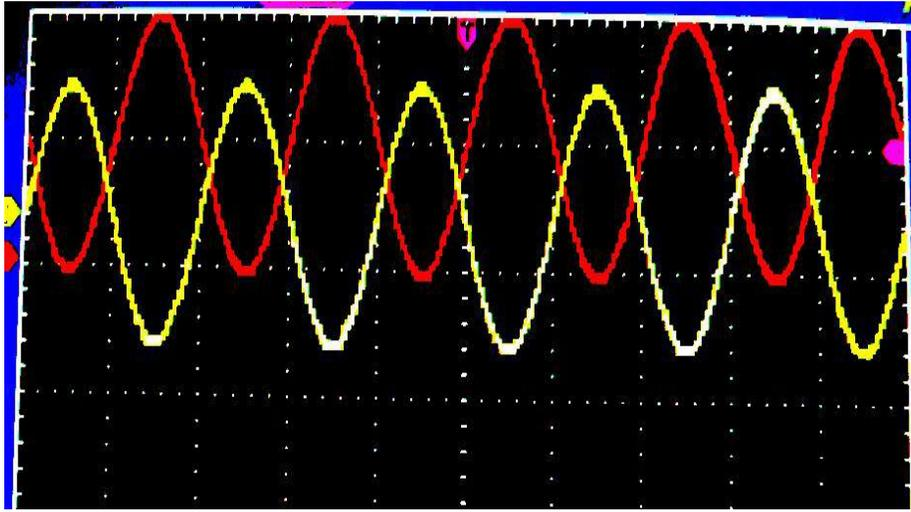
**Figure 6: Output of differential amplifier circuit**
