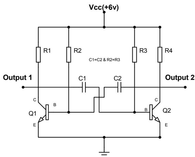
**Figure 1: Conventional basic astable multivibrator circuit**
