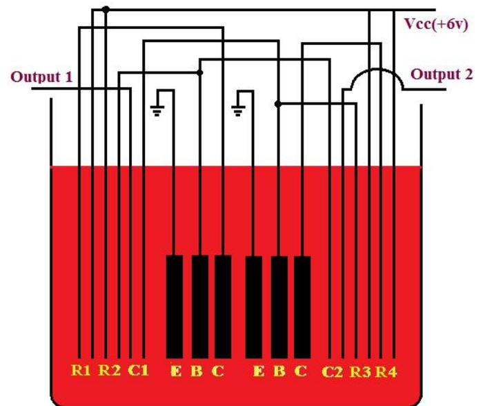
**Figure 2: Layout of liquid astable multivibrator IC**
