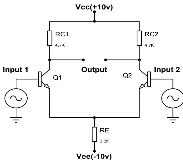
Figure 4: Conventional basic differential amplifier circuit
