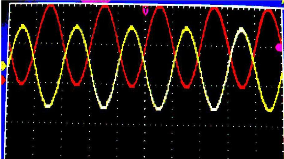
**Figure 6: Output of differential amplifier circuit**
