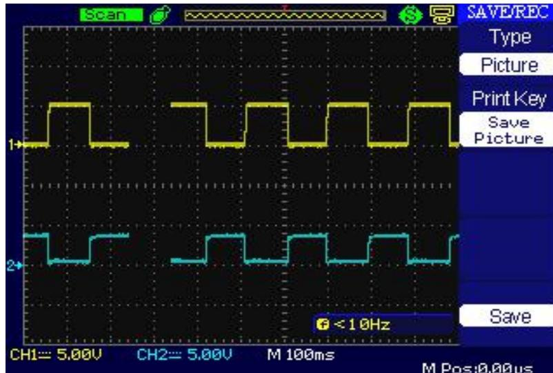
Figure 3: Output of astable multivibrator circuit
