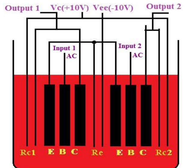
Figure 5: Layout of liquid differential amplifier IC
