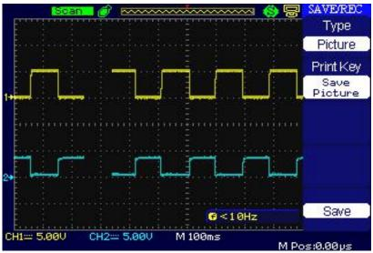
Figure 3: Output of astable multivibrator circuit
