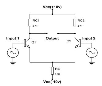
Figure 4: Conventional basic differential amplifier circuit
