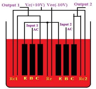
Figure 5: Layout of liquid differential amplifier IC
