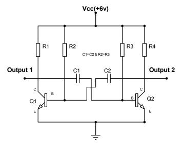
Figure 1: Conventional basic astable multivibrator circuit
